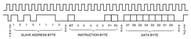
Figure 9. DCP Write Command Sequence
