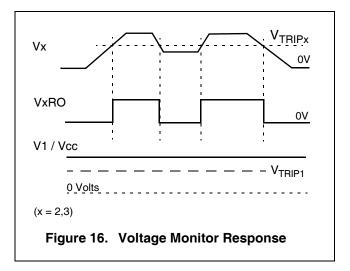
It is recommended to stop communication to the device while while V1RO is HIGH. Also, setting the Manual Reset (MR) pin HIGH overrides the Power-on/Low Voltage circuitry and forces the V1RO output pin HIGH (See "Manual Reset").
