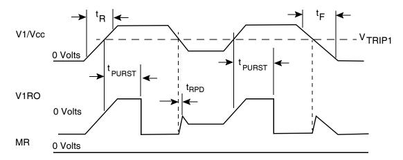
Figure 26. Manual Reset Timing Diagram
