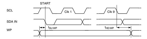
Figure 24. Write Cycle Timing
