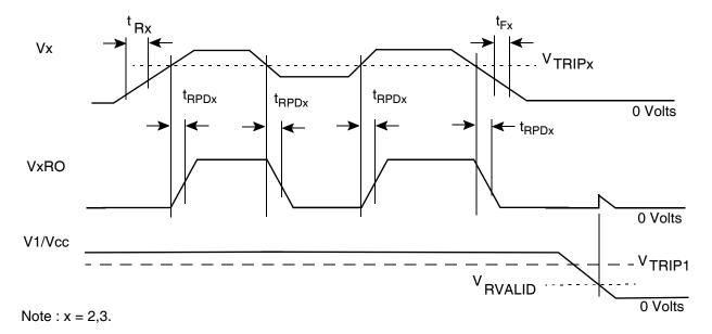
Figure 28.  $V_{TRIPX}$  Programming Timing Diagram (x = 1,2,3).
