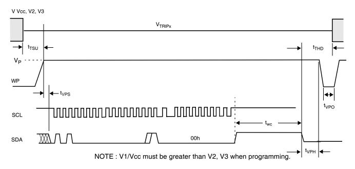
Figure 29. DCP "Wiper Position" Timing
