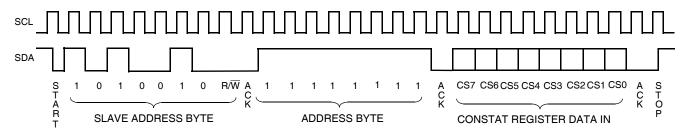
Figure 13. CONSTAT Register Write Command Sequence
