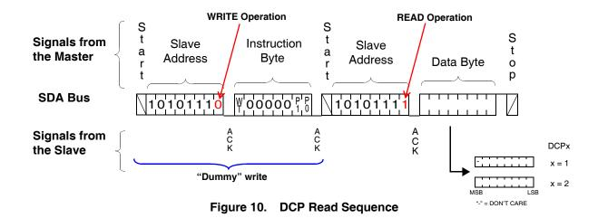
It should be noted that all writes to any DCP of the X9523 are random in nature. Therefore, the Data Byte of consecutive write operations to any DCP can differ by an arbitrary number of bits. Also, setting the bits P1 = 1, P0 = 1 is a reserved sequence, and will result in no ACKNOWLEDGE after sending an Instruction Byte on SDA.
